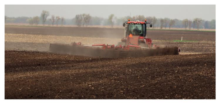
Counter-following design: The front and rear gangs on the TATU Speed Disk are positioned closer together compared to traditional disks, enabling it to closely follow the ground contours for improved depth control.
