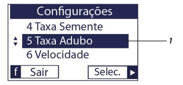
Screen F2 (1) indicates the fertilizer rate (2) in kg per hectare obtained with a specific gear ratio. Fertilizer rates are calculated according to the fertilizer calibration, the gear configuration (3) and the line spacing. The keys  $\nabla$  and  $\triangle$  (4) allow the user to navigate between the rate options in Kg / ha.
