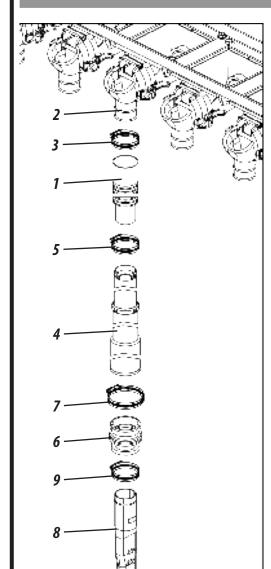
To send the fertilizer from the distributor to the ground, fit the hose (1) to the outputs of the independent conductor (2) through the clips (3). Then, attach the telescopic cable (4) to the hose (1) by attaching it through the clamp (5). Then, attach the rubber coupling (6) to the telescopic cable (4) by attaching it through the clip (7). Finish by attaching the spout (8) to the rubber coupling (6) by attaching through the clip (9).
