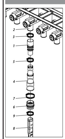
To send the fertilizer from the distributor to the ground, fit the hose (1) to the outputs of the independent conductor (2) through the clips (3). Then, attach the telescopic cable (4) to the hose (1) by attaching it through the clamp (5). Then, at ach the rubber coupling (6) to the telescopic cable (4) by attaching it through the clip (7). Finish by attaching the spout (8) to the rubber coupling (6) by attaching through the clip (9).
