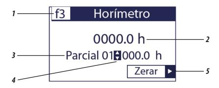
The F3 screen (1) indicates the total number of hours (2) of work with the ETD in three partials (3), which can be related to the keys  $\bigoplus$  (4).
