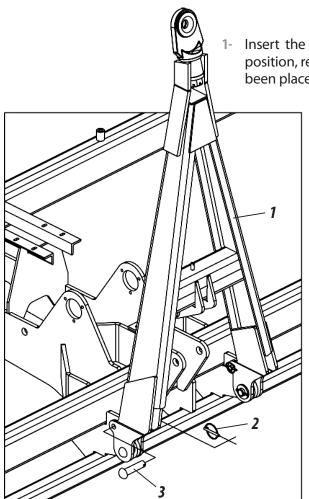
I- Insert the coupling head (1) into the working position, removing the (2), the pins (3) that have been placed for the transport of the seeder.
