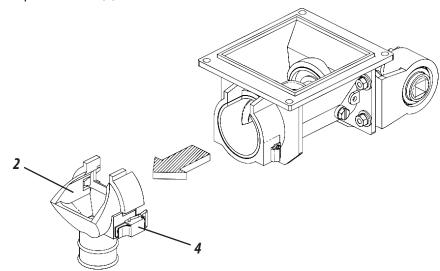
2- Then insert the maintenance tube (1) with rotating movements, promoting the movement of the fertilizer to the bottom of the doser. Then perform the necessary maintenance.
