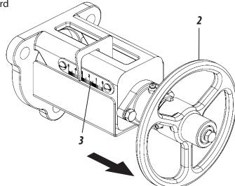
2- Then, turn the wheel valve (2) to the "A" or "B" direction by adjusting the doser (3) to the value found in the table on the following page, according to your needs and working condition.
