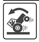
• Do not operate the tractor if the front is light. If there is a tendency to lift, add weights to the front or front wheels.
