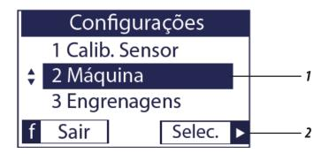
In the machine configuration (1), click on 'Selec  $\blacktriangleright$  (2) to inform the number of lines using the buttons  $\stackrel{\triangle}{=}$  (3).
