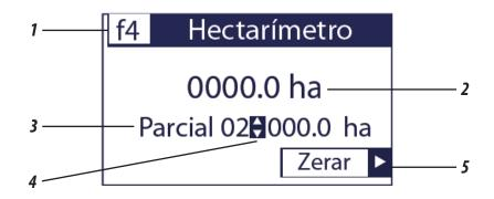
Screen F4 (1) indicates the total number of hectares worked (2) with the ETD, also in 3 partial ones (3), which can be selected using the keys  $\stackrel{\blacktriangle}{=}$  (4).
