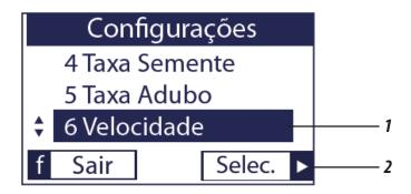
Clicking on 'Select.' ▶ (2) in the 'Speed' setting (1) will show how many hours (4) the machine has been working above the limit speed (3).
