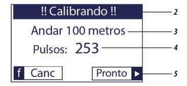
When starting the sensor calibration (2), the machine must be moved for exactly 100 meters (3) and stopped.
