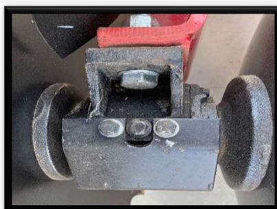
OIL BATH BEARINGS FOR EASY MAINTANENCE
