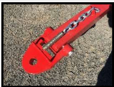
SIMPLE CHAIN AND SPRING ASSEMBLY ON HITCH ALLOWING FOR EASY HOOKUP
