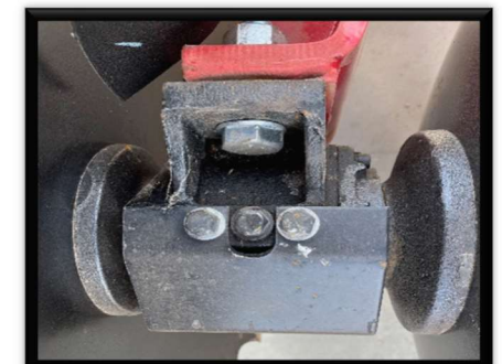
OIL BATH BEARINGS FOR EASY MAINTENANCE
