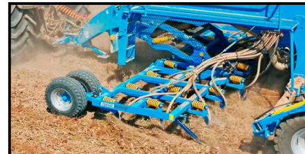
SHANK SECTION 24 shanks - 3 rows - 250mm spacing Allows for cultivation down to 200mm
