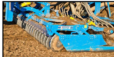
DISC SECTION 24x 490mm discs - 2 rows - 250mm spacing Allows for cultivation down to 100mm
