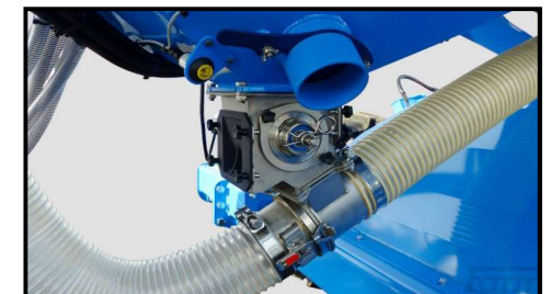
FARMET METERING SYSTEM with interchangeable rollers for different rates
