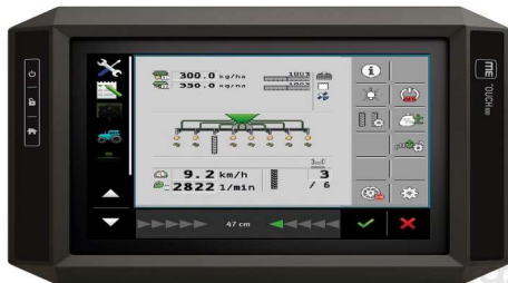
Müller Elektronik (ME) TOUCH800 In-cab ISO BUS Controller, 8" display
