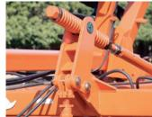
Front and rear gangs leveling are manually performed through stabilizer bar which controls the entire uniformity of disc harrow. Independent leveling adjustment rod threads are available on each wing of the harrow.
