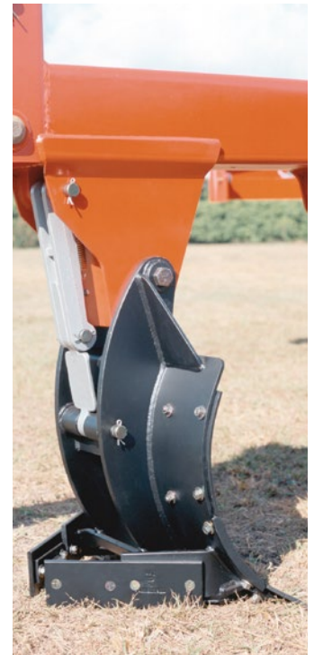
Moldboard trip system with flat spring
