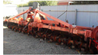
MASCHIO ZAPPATRICE 6m rotary hoe, double side gearbox, 1000 PTO, safety guards, oil cooler, hardened blades, rear tool bar. $24,250 inc GST
