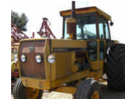
CHAMBERLAIN 4480 125hp, rear duals, rear weights, A/C Cabin, 540 PTO, draw bar, no linkage,
